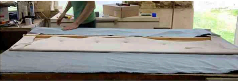
Spray glue on to foam, put on the fabric/smooth down, turn over
